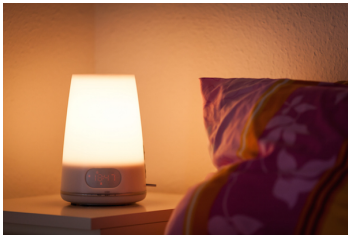
Figure 1: This alarm clock uses ambient light to softly wake up its user. We envision that it could also be used as a helpful output device for other information, e.g., incoming phone calls or reminders.
